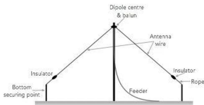
Basic inverted V dipole antenna concept
