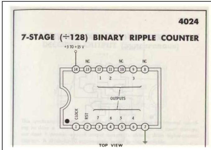
This is a binary ripple counter that counts in the up direction using positive logic.
